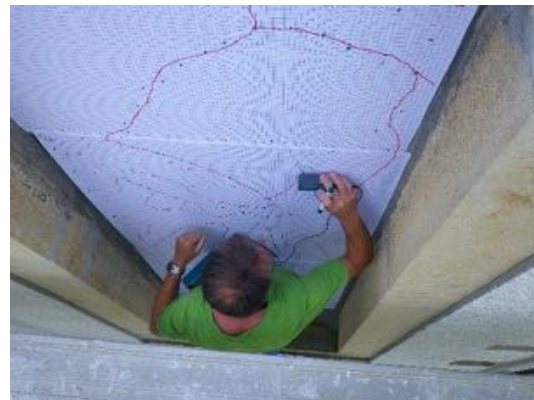
Abbildung 22: Profometer5+ in Courfaivre
